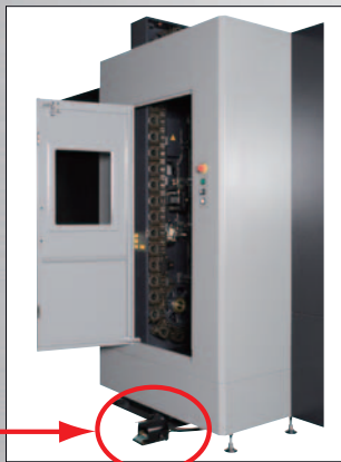
Foot-operated switch for removing a tool (Standard)
